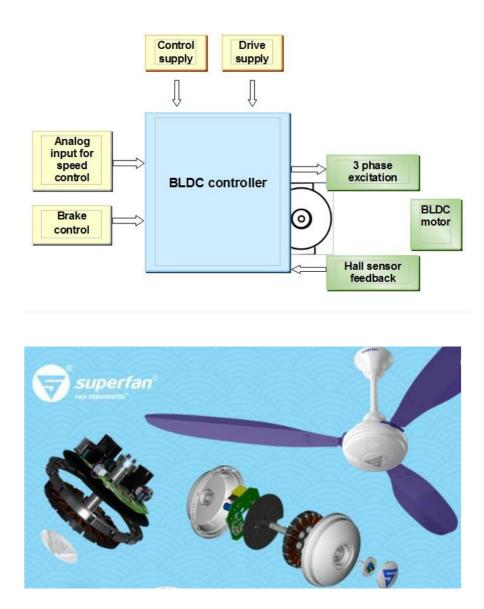
With the replacement of existing ceiling fans with Super Fans the energy consumption is likely to reduce by 55% per fixture. Considering 100 fans being replaced with super-efficient BLDC fans, 3.50 kW can be saved.
